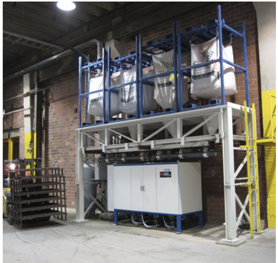
An ACT Würschum COM 70-3 granular color pigment metering system features closed-loop pneumatic dispensing from three separate conveying vessels for dust-free operation.
