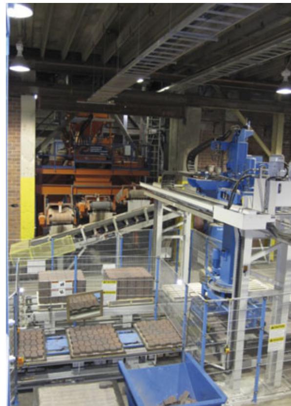
The ACT MobilMat Mo80 turnkey concrete batch plant (in orange) supplies the Hess Multimat RH 1500-2 paver production system (foreground) at the Shaw Brick facility in Lantz, Nova Scotia. This new plant investment was made economically attractive by housing it in a "vintage" building that was given a cost-effective makeover.
