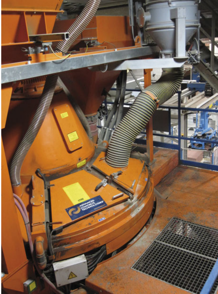
Shaw Brick's ACT MobilMat Mo80 batch plant features the HPGM 2250 high shear planetary counter-current mixer (shown above on raised platform) equipped with the ACT Hydromat microwave water metering system for consistent water/cement ratio adherence.
